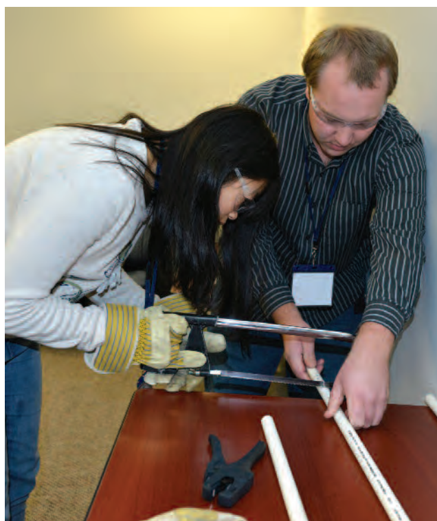
Student wears safety gloves and glasses while sawing a PVC pipe held by instructor
