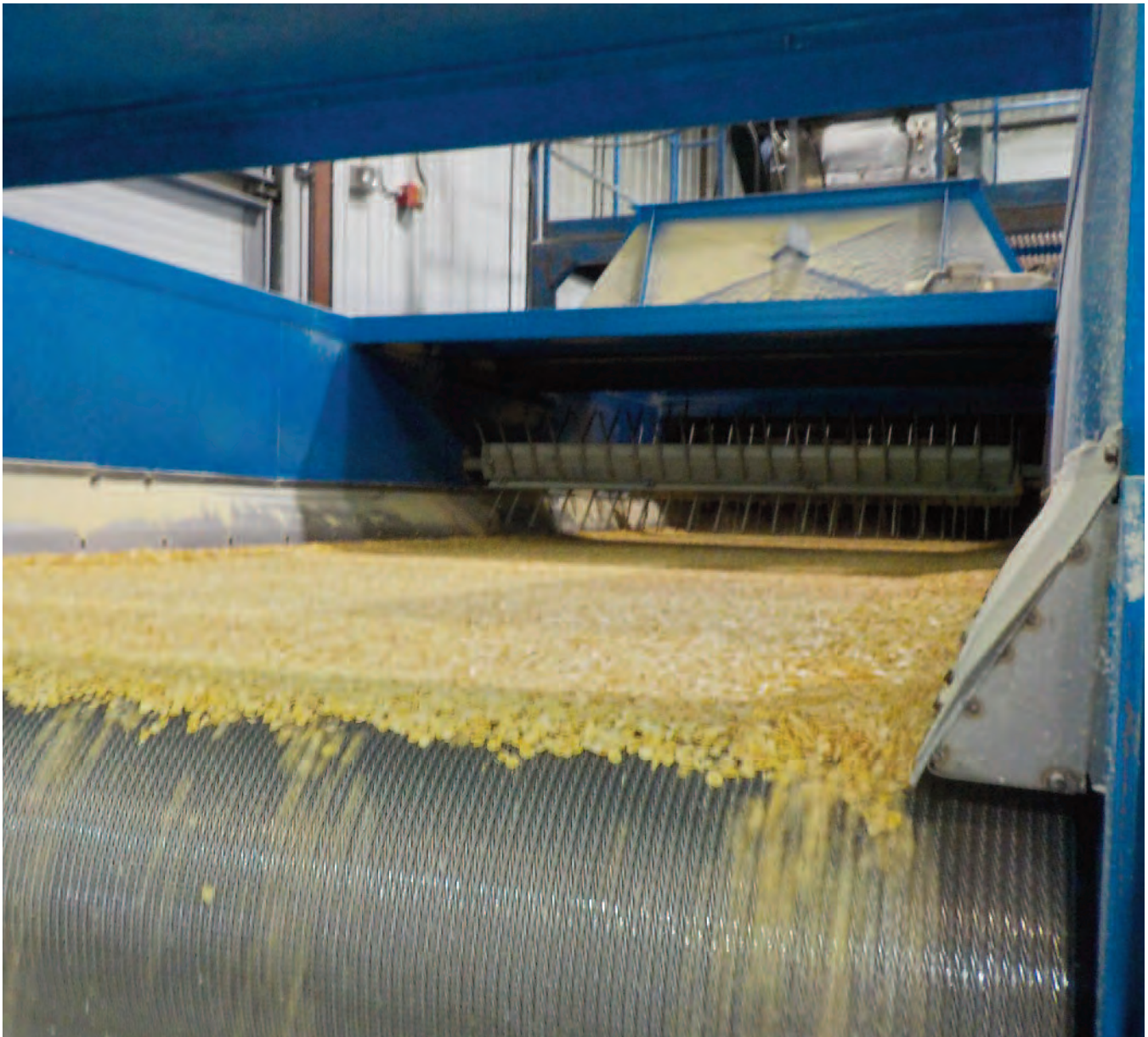
Hundreds of tonnes of pulses travel through an assembly line before they reach the bagging stage. PAMI engineers designed custom-made conveyors to allow the pulses to move down the line.
