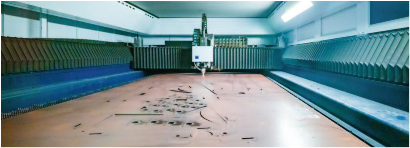
Smart factory laser: Brandt's smart factory is home to three 10-kilowatt fibre lasers. Two of these lasers are connected to PartMaster manual sorting stations, while the third employs a fully automated SortMaster to pick and stack parts.
